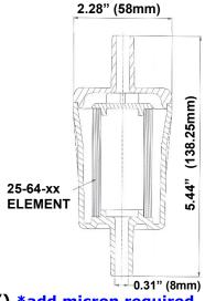
Large OEM Maximum Flow DIF with SS Screen (DIF-LN\_SS-1/4") \*add micron required
