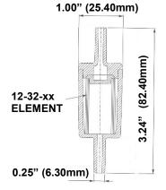
Standard OEM Size with Stainless Steel Screen (DIF-BN\_SS) \*add micron required
