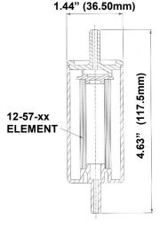
Intermediate OEM High Flow Coalescing DIF (DIF-IN\_\_C) \*add grade required
