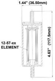
Intermediate OEM High Flow DIF with SS Screen (DIF-IN\_SS) \*add micron required
