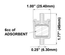
Intermediate OEM High Flow DIA w/ Media (DIA-IN) \*add adsorbent required
