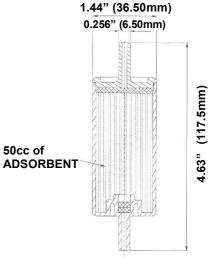
Large OEM Maximum Flow DIA w/ Media (DIA-LN\_\_) \*add adsorbent required
