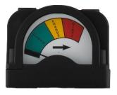
The Visual Differential Indicator is designated as "VDI" and is designed as a colored gauge with set points from 0 to 5 PSIG in the green range, 6 to 9 in the yellow range, and 10 to 14 PSIG in the red range.
