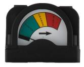
The Visual Differential Indicator is designated as "VDI" and is designed as a colored gauge with set points from 0 to 5 PSIG in the green range, 6 to 9 in the yellow range, and 10 to 14 PSIG in the red range.
